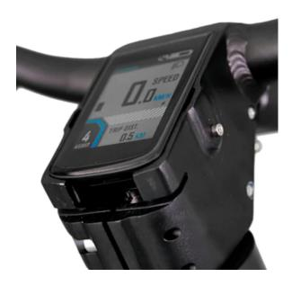
BC281 display uses independent press button, in total five buttons:
